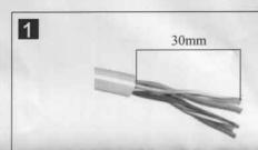
Strip approximately 30mm of the cable jacket, and separate to 4 pair each.
